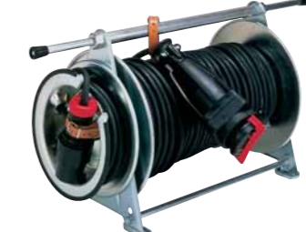
Cable drum, with 100m H07RN-F5G1,5 Width of winding 440mm Dimensions (wxhxd) 310 x 377 x 573 mm Weight approx. 58 kg
